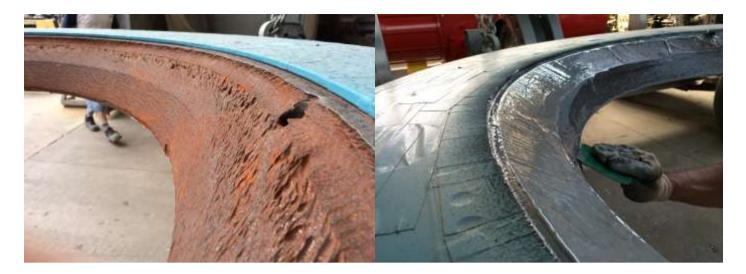
Resimac manufactures a range of solvent free epoxy repair products that contain hardened ceramic beads.
